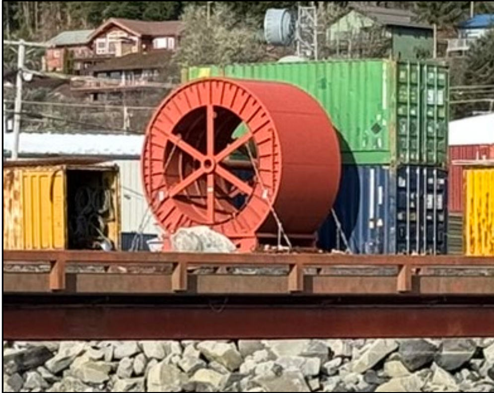
FIGURE 21. Steel electrical cable spool; weight estimated to be over 40 tons.
