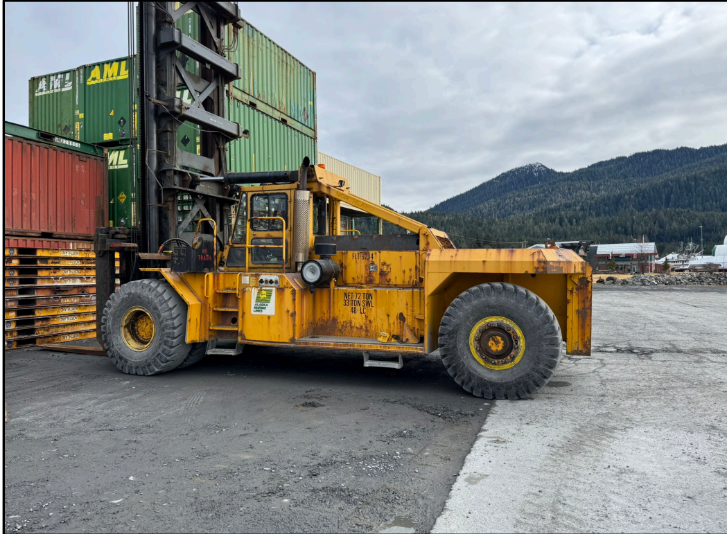
FIGURE 18. Forklift used for handling freight; 77 ton weight; 33 ton safe working load.
